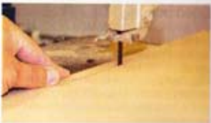
▲ Pic. 2 The template is trimmed back to this line using whatever method you have to hand, such as bandsaw, coping saw or jig saw
