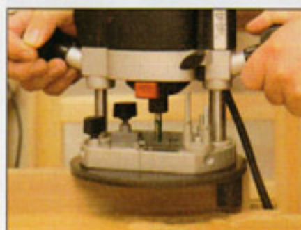
The cutting action of the router keeps the cutter centred
