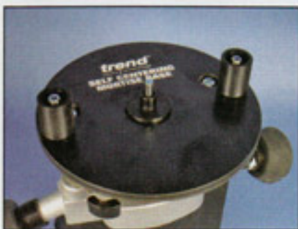
The base is centred using the centring device supplied
