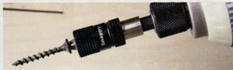
Here the bit is set to drive under the surface while still holding the screw
