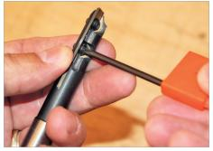
A couple of Torx screws retain the cutter using a supplied wrench
