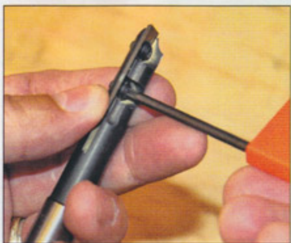
...and is held securely in place by two small Torx-head screws
