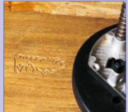
Checking the first element of the design routed into an iroko sheet with the Routasketch
