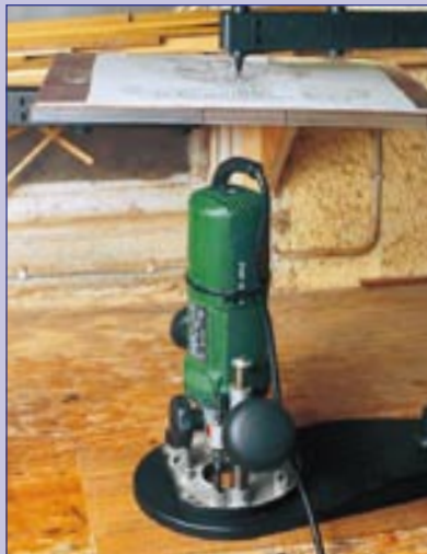
As the cable entry on the little Bosch router exits at the top of the motor housing, a cable tie keeps the mains lead from fouling the underside of the drawing table
