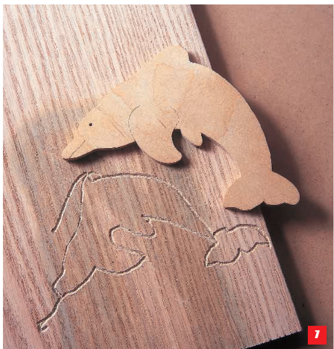
This is what happens if the drawing carrier plate moves
