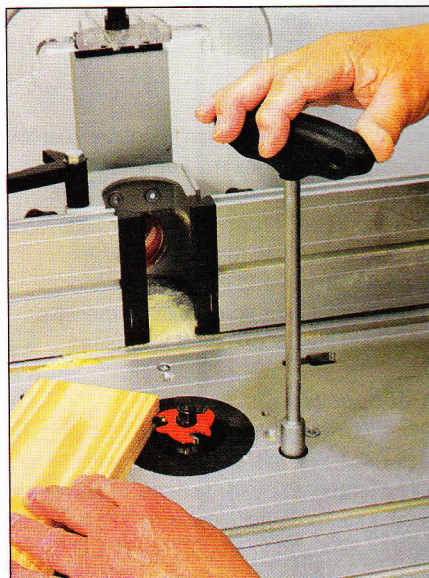
The Trend T11 in the PRT table showing above-table height adjustment
