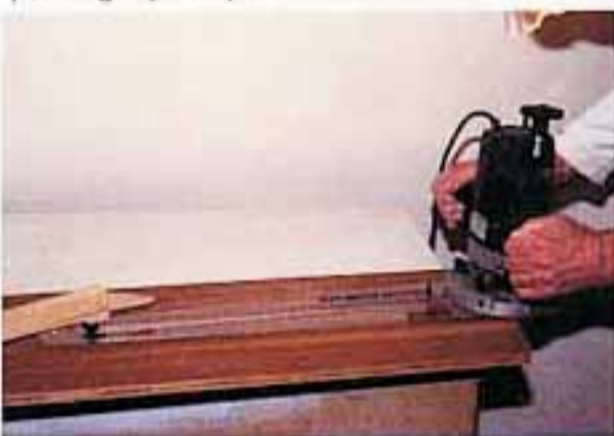
Trimming a curved end. Note the compass point lightly clamped to the wood.
