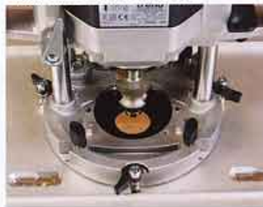
Quick release fittings on Trend table with T11 router
