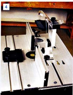
The guard assembly lifted by the pivoting rectangular section tube
