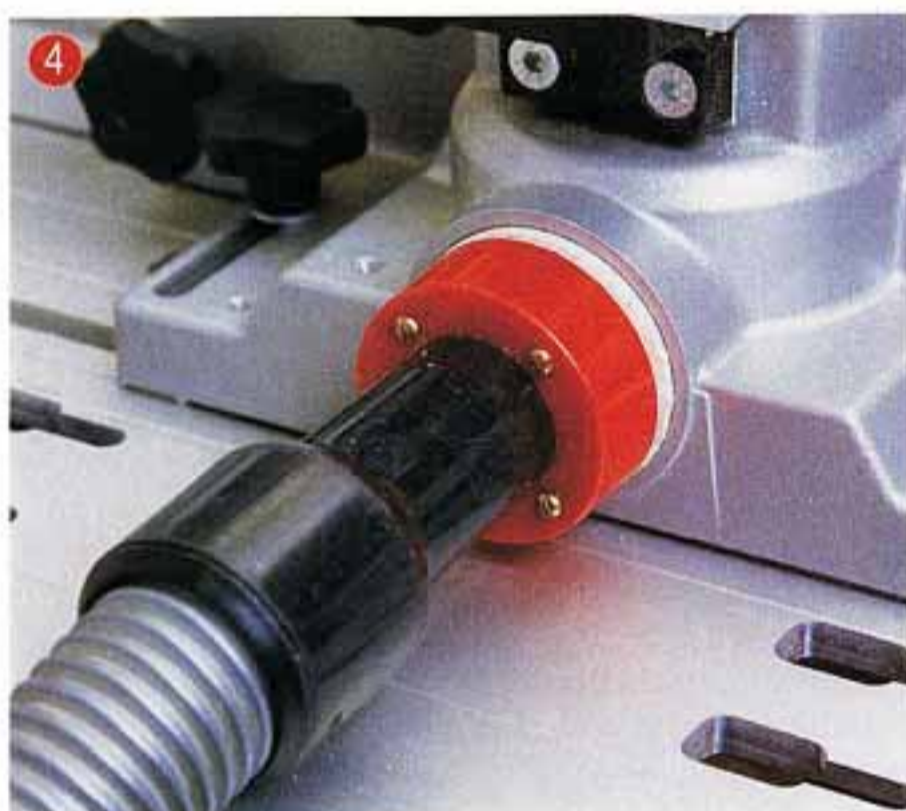
The dust extractor connected with a home-made adaptor
