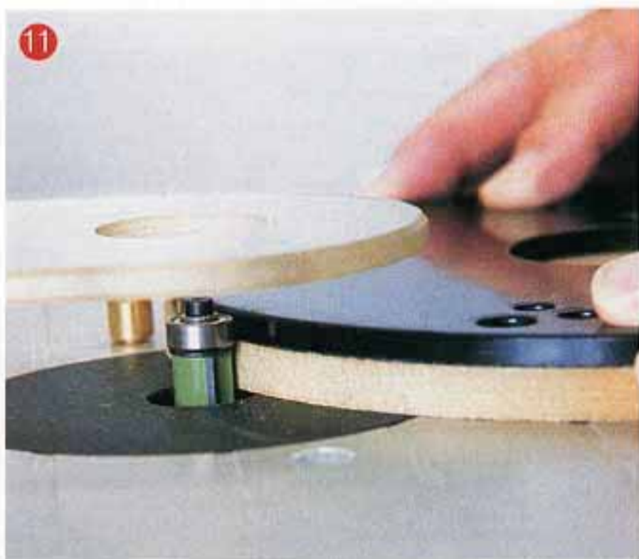
A base pattern in MDF being made for the Bosch 2000 router
