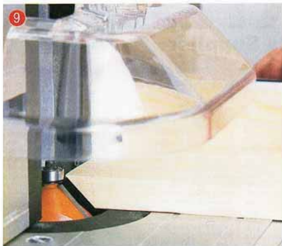
The ends of a box component being mitred
