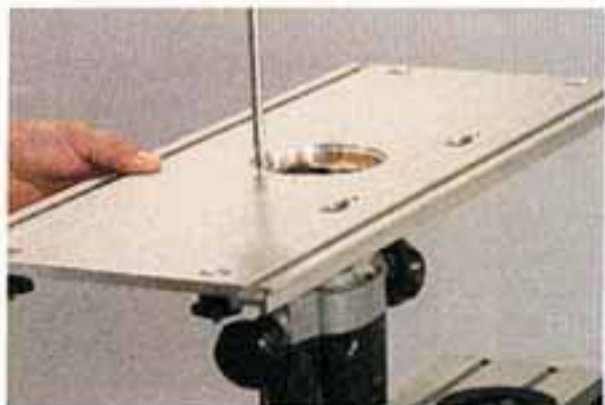
Router mounting is simple with the centre section of the table removed.
