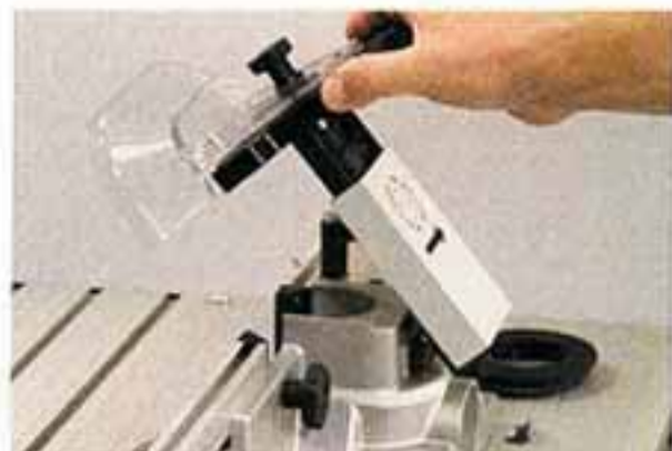
The Perspex guard hinges back for better access.
