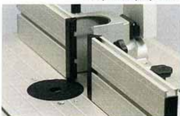
The fences are properly true but not independently adjustable.
