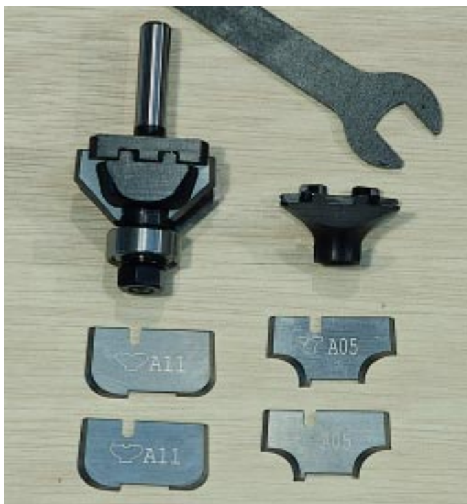
Clockwise from top: Locking nut spanner; cage for concave blades; pair of round-over blades; pair of cove blades; assembled cutter (with chamfer blades fitted)
