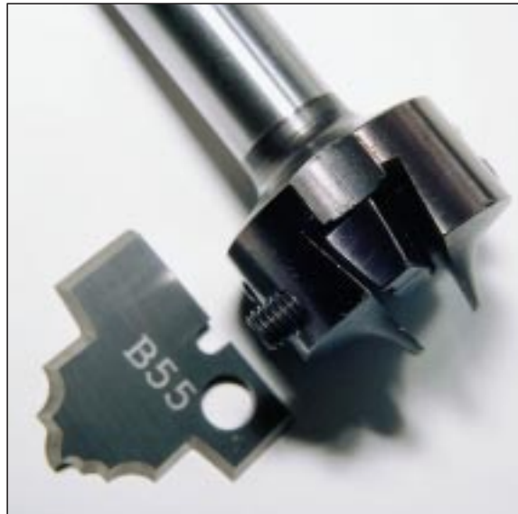
Type 'B' body blade removed, note locking wedge
