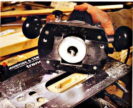
Setting up the template for the tenon
