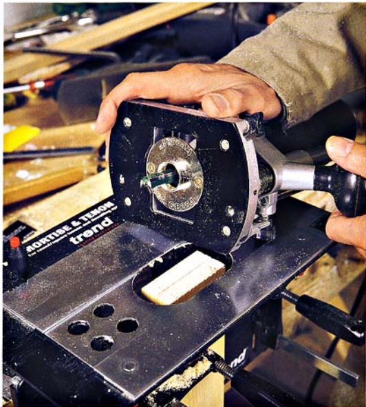
Ready for routing the tenon
