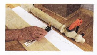
a convenient way to mark out circles from 1" to 19¾" in diameter. Thread a string, and the trammel transforms into a nicely-weighted plumb bob. With the string still in place, rotate the head 90°, and the bob turns into a line block or, with the addition of chalk, a chalk line. (This might seem like a stretch, until you try doing these jobs without a helper.)
