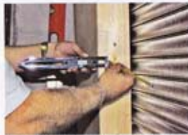
▲ Pic. 5 The Multiscribe can be used for other things such as general marking out for hinges, for example
