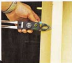
▲ Pic. 1 You can alter the setting so that the pencil is in the correct position for the amount you need to remove. This particular setting is to get a panel flush with the edge of a stud when scribed against a stone wall in the workshop
