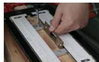
With the case routed and the jig still clamped, the stops are then adjusted
