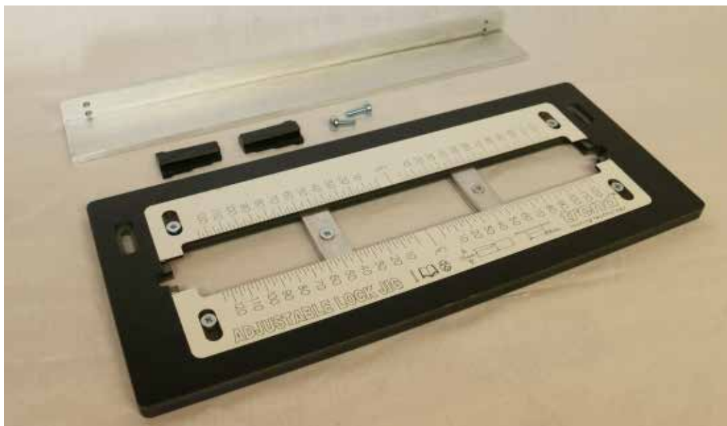
The underside of the jig is etched for common door widths to centralise it on the work
