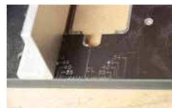
The underside of the jig is etched for common door widths to centralise it on the work
