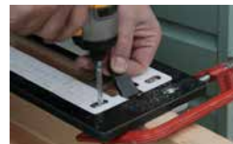
A pair of spacers is supplied to set the width for common lock case and faceplate widths
