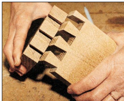
Photo 4 After machining the two halves, simply open out, book fashion
