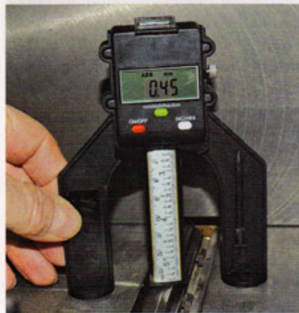
The Digital Depth Gauge allows you to work in either imperial or metric units
