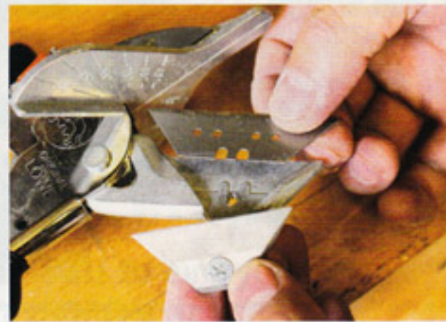
▲ Blade swapping is a very easy operation
