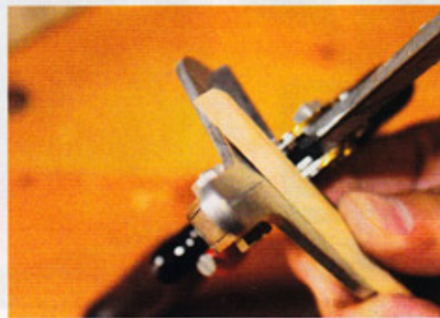
▲ You can see the tilt of the beds to try and counteract the work sliding back
