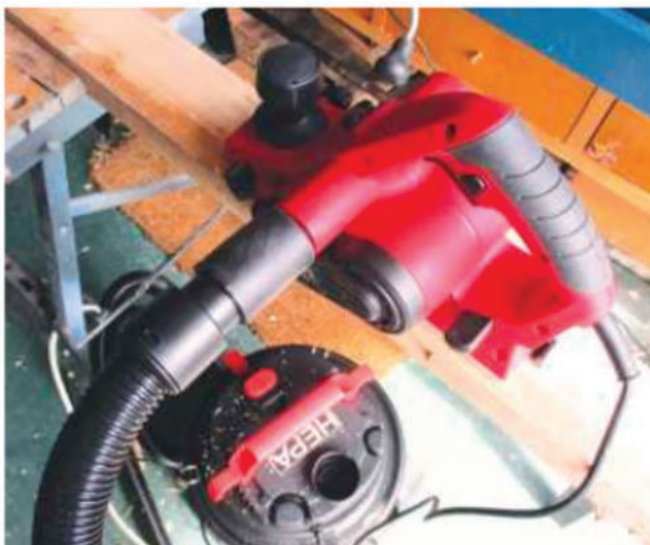
A flexible dust spout adaptor provides dust control on a planer...
