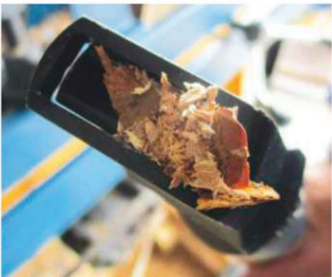
The crevice tool can get blocked with bigger chips
