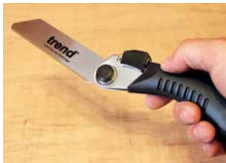
▲ ...or cranked back, ideal for working into a tighter area
