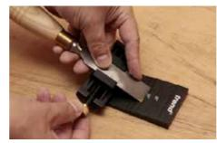
A You slide the blade through until it rests against the ridge of the required hone angle
