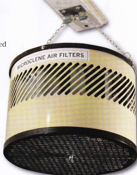
The Microclene ambient air filter hanging from the workshop ceiling
