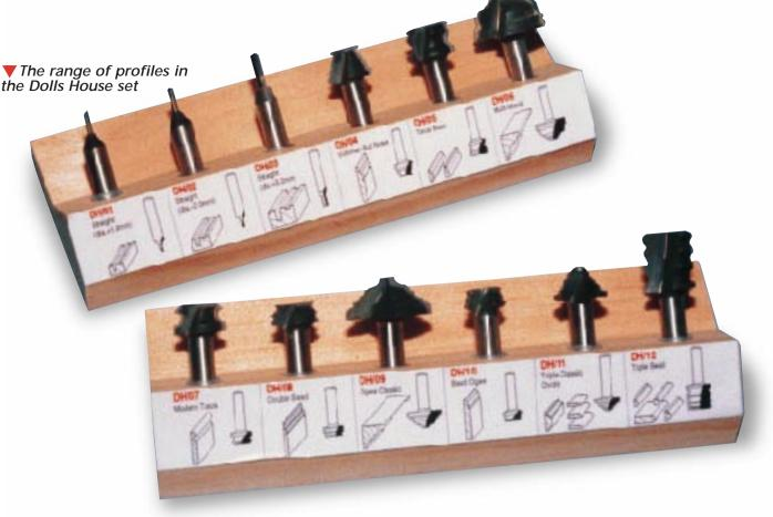
The shape produced simply depends upon the cutter's height above the router table. Therefore, an individual cutter such as the multi-mould can produce beads, dart cornices, covings, cornices, ovolo moulds for furniture, skirtings, architraves and picture frames. In order to rout a picture frame a straight cutter is used afterwards to form the rebate.
