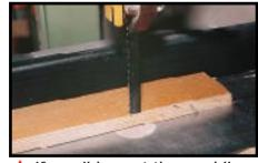
▲ If possible, rout the mouldings on a larger piece of wood then saw them off
