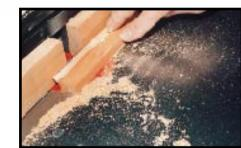
A router table is essential for machining small mouldings like this cornice
