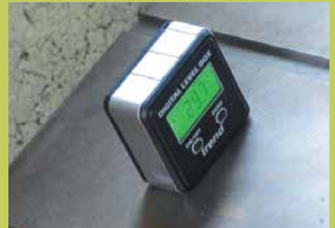
Its tough alloy rim has a magnetic base so will attach itself happily to steeply tilted, vertical steel or cast-iron surfaces
