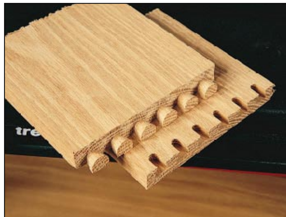
▼ The finished dovetail joint ready for assembly
