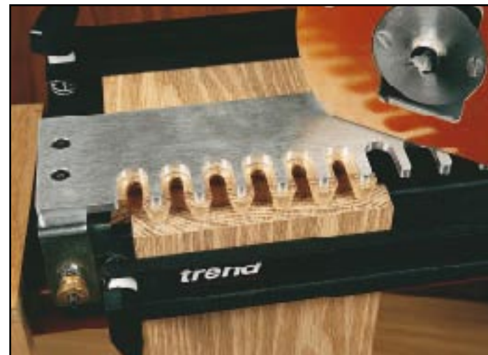
▲ Clamp the workpieces into the jig, inside faces out
