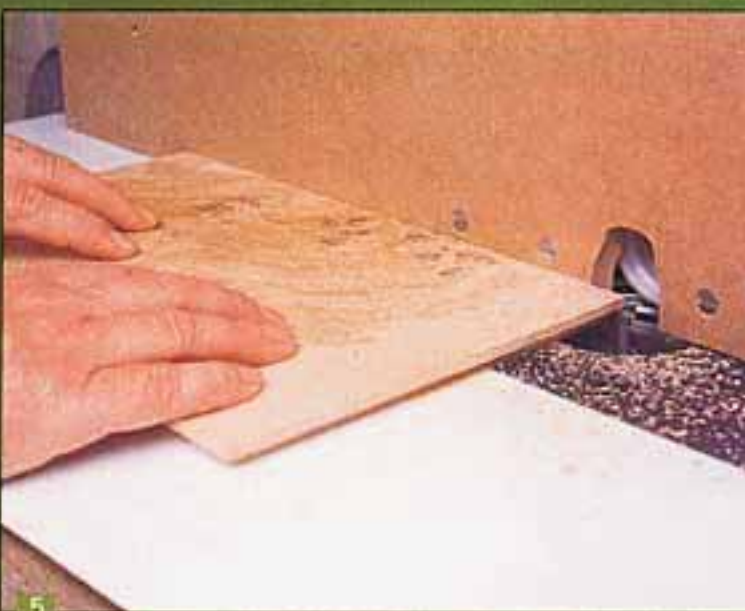
5 Cut a rebate around the top and base panels
