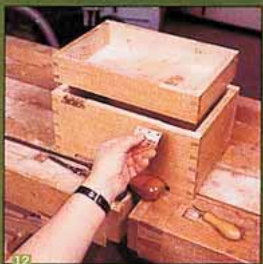
12 Hinges being positioned
