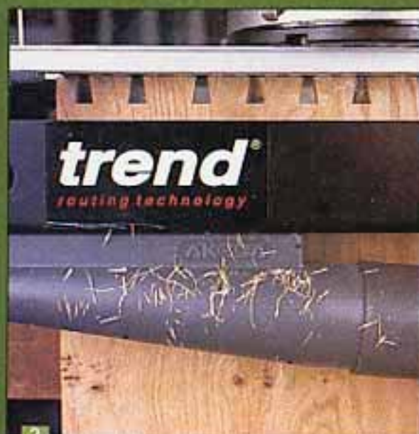
2 Cutting oak dovetails on the jig
