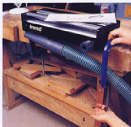
Clamping down the baseboard
