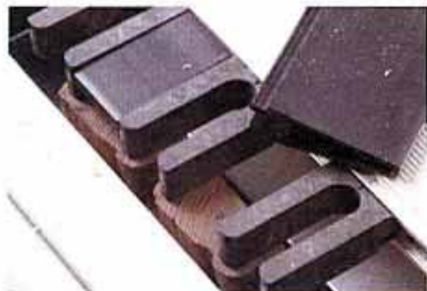
... but you can buy spacers that can be cut to fit between fingers on widely spaced dovetails.
