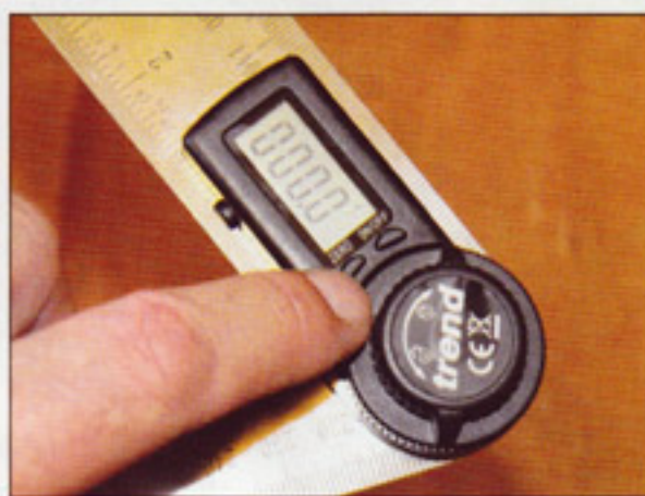
This button allows you to zero the setting with the blades at any angle
