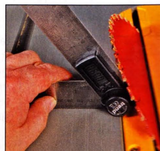
Setting the tilt angle on a table saw
