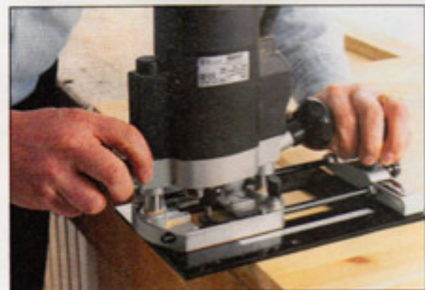
4 The offset base totally eliminates any risk of the router tipping in use
