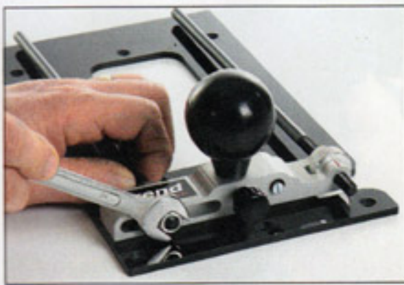
2 Different bar-hole spacings are accommodated simply by moving one of the bars
