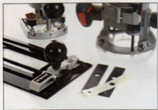
1 Shims lift the bridge to match the height of your router's bar holes
