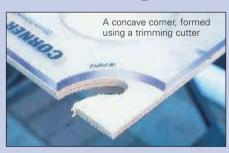
However, a little care is needed to ensure that the height settings are correct, or there is a danger that the cutter can also cut the template.
