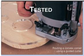
mongst the new items to be featured in Trend's latest routing catalogue are a number of templates in tough, clear PETG plastic. One of these is for use when forming rounded corners as well as holes and circular recesses. This template measures 290mm x 290mm and is 8mm thick.
