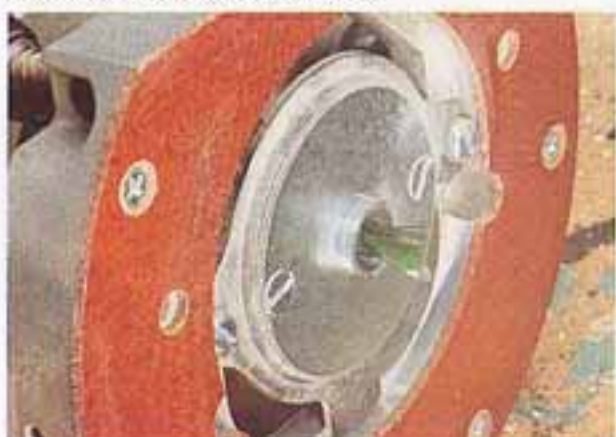
To use the jig, a guide bush needs to be mounted into the router base.
