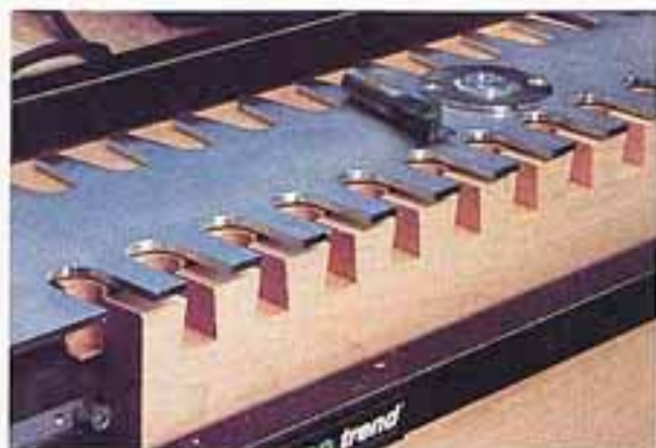
...while tails are cut with a dovetail bit on the other side of the comb.
