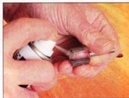
Protecting the cutter with PTFE dry lubricant will stop resin build-up
