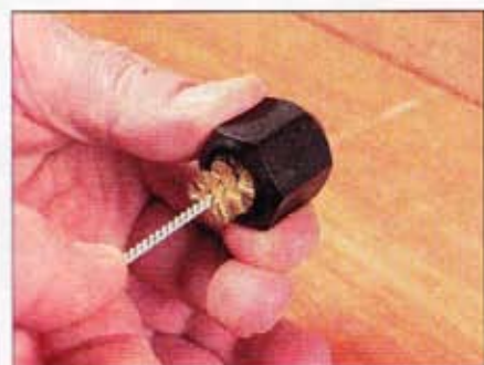
The wire brushes are ideal for cleaning the threads inside the collet nuts
