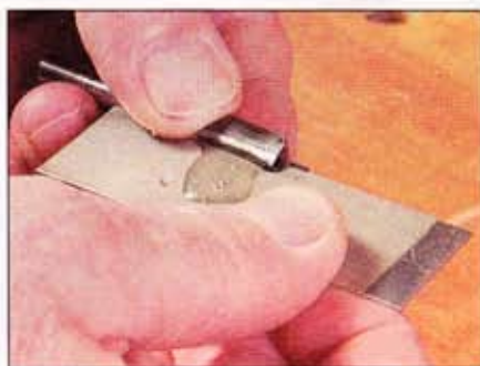
Lubricating the diamond card using the Rust Buster lubricant
