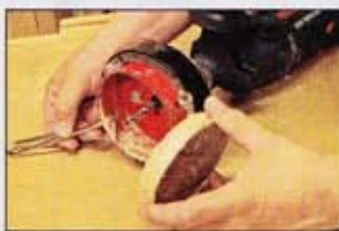
Remove the blank while the saw blade is still hot
