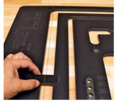
▲ The jig comes with a datum gauge block to correctly set it up to the layout lines
