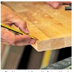
▲ The drip groove is formed by first marking the backset start and finish point for the cut
