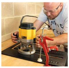
▲ The cut is made in two halves, working from the left inwards to avoid breakout
