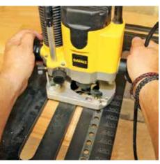
▲ With the jig set and clamped for the drip, the first cut is made
