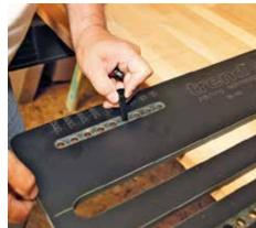
▲ Specific backsets can be set using the supplied pins
