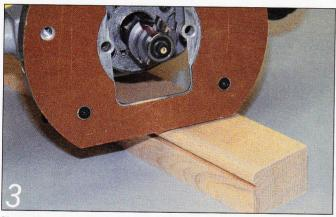
Plunge the cutter and use the locking handle on the router to secure this in position before making the cut. Profile the edge of the timber, working from left to right and moving the router at a steady speed to avoid burning the wood. Avoid plunging the router into the timber or out of it. Instead start the router while the base is positioned on the wood but with the cutter held away from the wood. Then feed the cutter into the wood and make the pass
