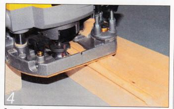
Depending on the job in hand, this step could complete the moulding. However, the clever bit is to turn the timber through 90° onto its side and to make a second pass so the two mouldings join together. The result is the effect of a bead cut onto the corner of the wood. For best effect it is important to set the depth of cut very precisely, and it's worth testing this on a scrap piece of timber first
