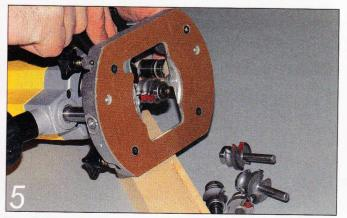
When fitting the cutter, ensure that at least two thirds of the shank is held in the collet and that the securing nut is tightened fully. Set the depth of cut carefully. The cutter being fitted here cuts two reads alongside each other, and when the cuts are joined they make an attractive corner feature
