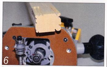
Four different cutters were used two produce these effects. The Trend cutter previously mentioned makes the attractive shape shown on the top right-hand corner of the timber, while the two simple beads are made by two similar cutters of different radii. This double reed effect is a useful method of decorating small table legs. You can create a different effect if the cutter is plunged deeper and the reed is run down the centre of the leg
