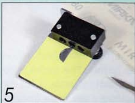
5 Stick fine abrasive paper to the jig to give it a non-slip surface
