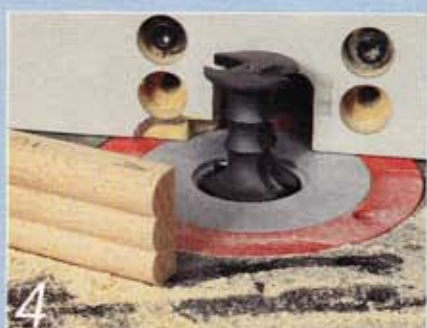
4 Reverse the piece to complete the moulding
