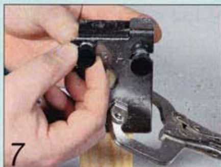
7 Reposition the jig and drill the intersecting holes
