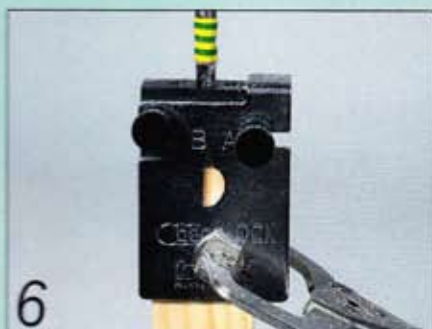
6 Clamp the jig in place and drill the first set of holes
