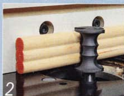
2 Use a piece of kit tenon to set up the router
