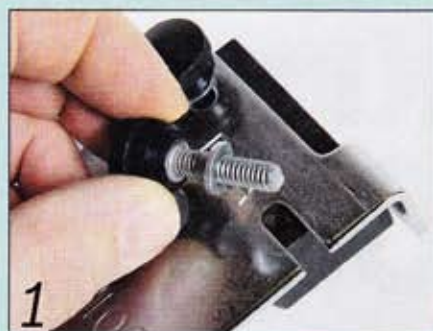
1 Add washers to the knurled knobs to make them easier to tighten
