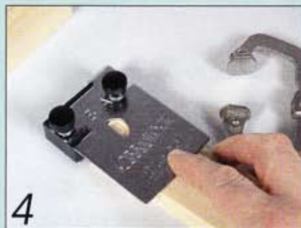
4 Align the mark on one piece with the D-shaped cut-out in the jig
