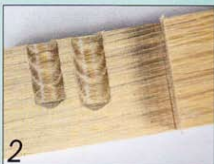
2 The higher the drill speed, the cleaner the hole; use a sharp drill
