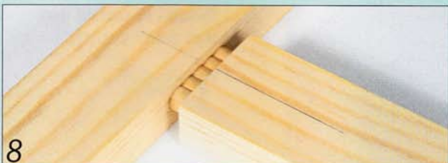
8 Insert the glued tenon, then assemble and cramp the joint
