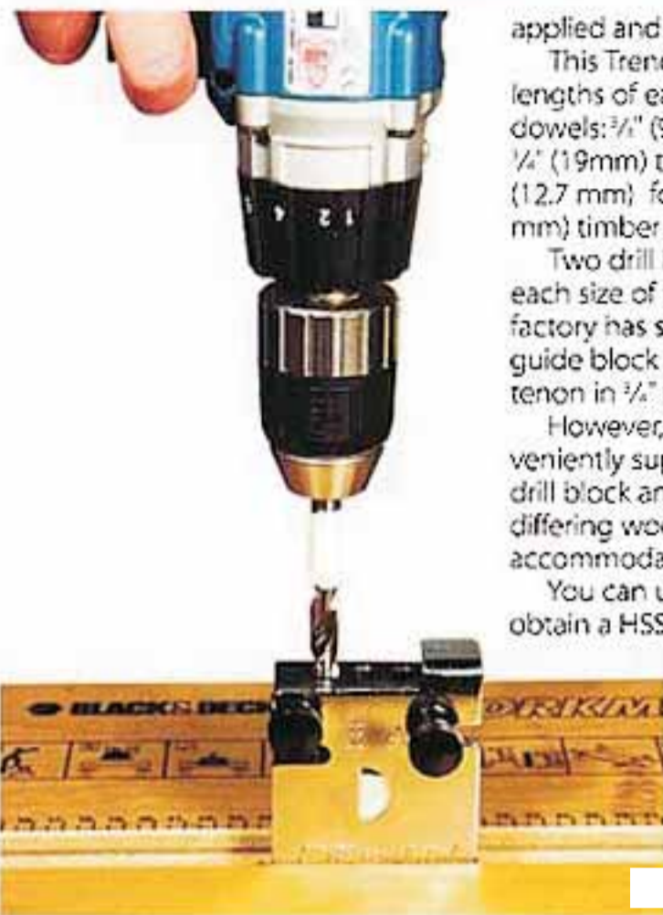
The work and the jig is clamped so that the mortises can be drilled. A piece of tape around the bit gauges the depth
