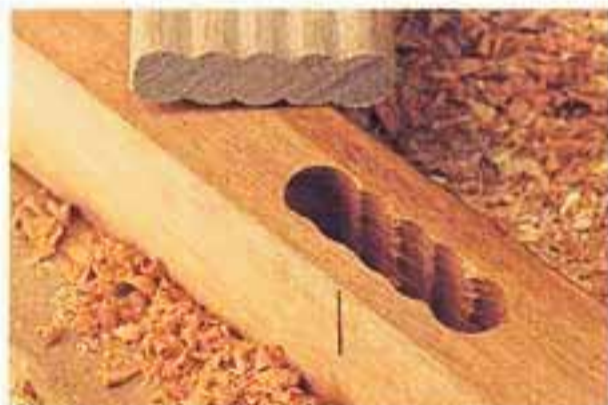
The finished Beadlock mortice and tenon material.
