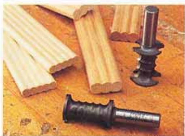
Router cutters are available for making your own beaded loose tenons.
