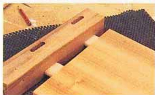
Use two joints for wide jobs which can be offset for non central fixing.
