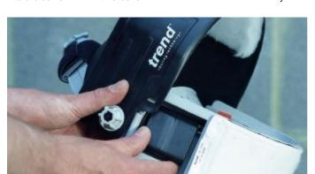
Batteries are rechargeable, and take just a second or two to fit in the sidemounted holder. Useful life is four hours on a full charge, but there is a second holder on the other side to let you double this by adding another
