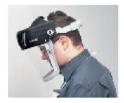
Respiratory protection is provided by a pair of renewable filters that will trap fine dust. It is also suitable for use with water-based aerosols. A flow meter is included, to ensure that sufficient air is passing through the system, and to warn when the filters are becoming clogged.
