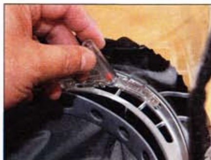
This tube fits over the air port to show how much airflow is getting through
