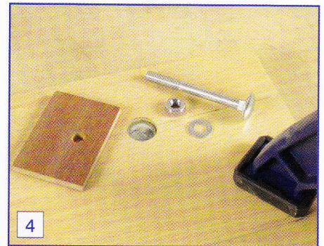
4 A pad of wood used under the bench top to act as a spacer when the nut is in place
