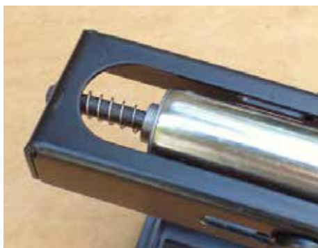
The polished steel roller is 250mm long, springs at either end of the shaft enabling it to move lengthways as well as rotate
