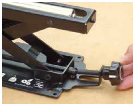
Working on a similar principle to a car scissor jack, you rotate a plastic knob at one end to raise or lower the screw mechanism
