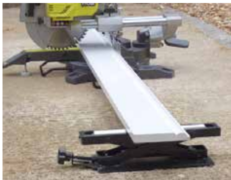
When cutting long timber lengths, boards often need to be supported at the farthest end from the blade
