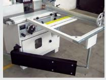
The optional table extension enables larger sections to be machined easily.
