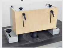
The optional tenoning hood is suitable for use with larger diameter tools (up to 300mm diameter).
