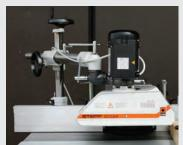
An essential piece of equipment on any spindle moulder. It provides a good finish on the material due to a constant feed speed and is the safest way to profile on a spindle moulder. The power feed comes complete with 3 rollers and 4 different speeds. It connects directly to a 3 phase socket at the rear of the machine. Horizontal arm measures 1050mm.
