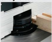
The optional alloy safety fence has individually adjustable sliding fingers that can be locked in position around the cutter heads. It provides good support to the workpiece when profiling and prevents it from 'dropping in'.
