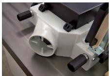
The back fence has an integral micro-adjuster which controls the position of the complete back fence.
