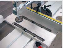
The 20mm thick tenoning table fits easily into the slot on the sliding table. Used in conjunction with the tenoning clamp and fence; suitable for getting smaller workpieces closer to the cutter heads.
